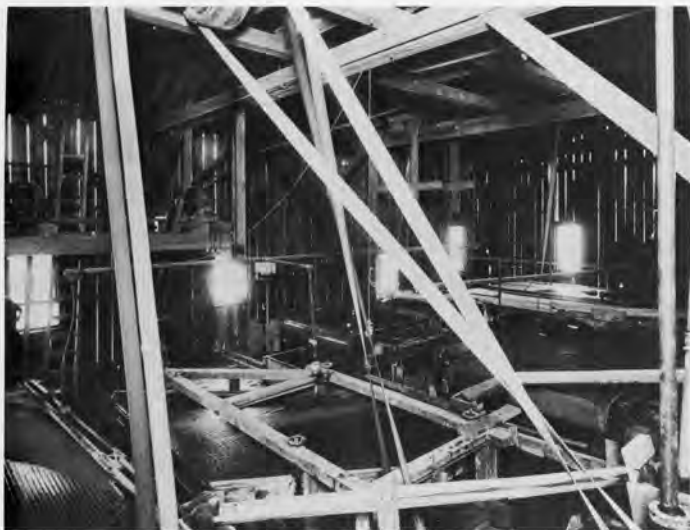
FIGURE 4—Shaking tables (left foreground) and slime concentrating tables (right) in Vanadium Mines Company remodeled mill. The slime tables were a recent development and may have been the source of considerable concentrate loss. Photo courtesy Mrs. Lydia Key, Black Range Museum, Hillsboro.
