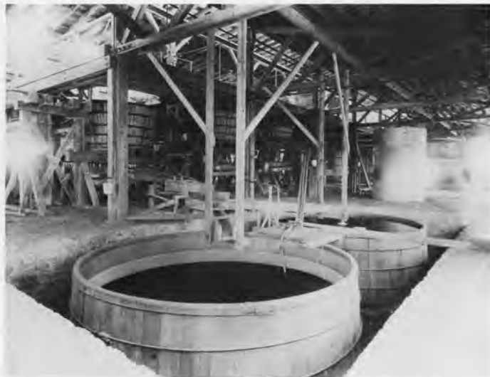
FIGURE 6—Vanadinite concentrates were leached with sulfuric acid in the upper tanks; the vanadium-sulfate solution was then decanted, probably to the holding tanks, foreground, from where it was taken, apparently by hand, to an evaporating furnace followed by calcining to V_2O_5 . Photo courtesy Mrs. Lydia Key, Black Range Museum, Hillsboro.
