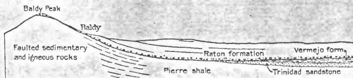
FIGURE 20.—Sketch profile through Baldy Peak and Aztec mine, Baldy, N. Mex., showing the unconformity between the Raton formation and the Pierre shale. The gold ore at Baldy occurs along this unconformity.
